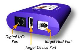
Figure 19: Beagle USB 480 Protocol Analyzer - Capture Side
