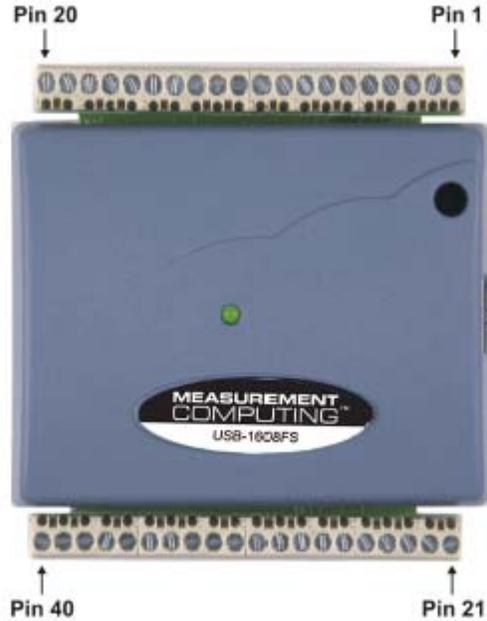
Figure 3-2. USB-1608FS screw terminal pin numbers
