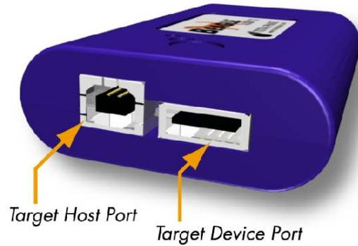
**Figure 23:** Beagle USB 12 Protocol Analyzer - Capture Side
