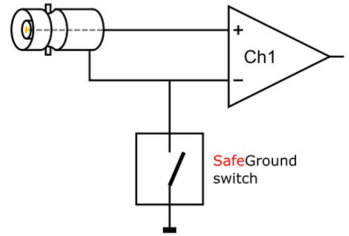
**SafeGround** protects your scope, your computer and your circuit under test against accidental wrong ground connections.
