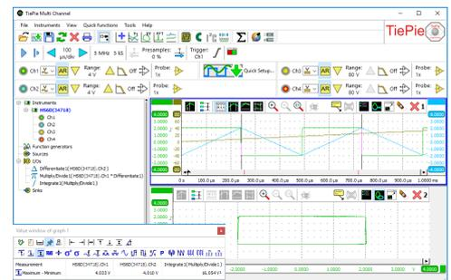
This measurement determines the area of an XY graph, using multiplying, integrating and differentiating I/O's. The area is indicated in the Value window: 16 V<sup>2</sup>.
